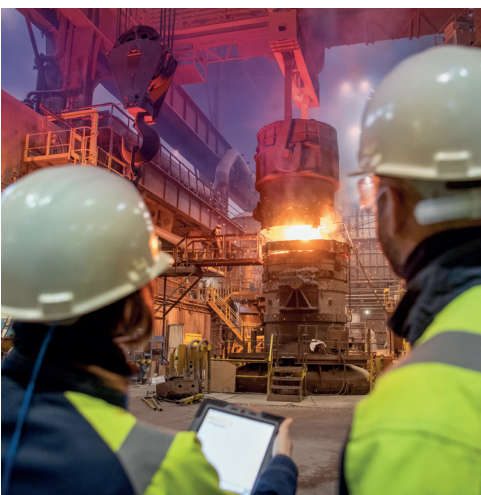
Fig. 4 Steel casting ladle
