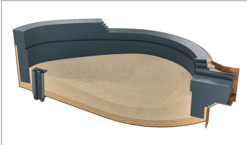
Fig. 2 Electric Arc Furnace (EAF)
